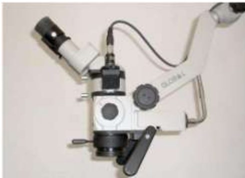
Fig. 32.11. Inclined binoculars. The inclined tubes are fixed at 45°.
