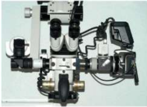
Fig. 32.14. Leica microscope fitted with the inclinable binocular, beam splitter, documentation adaptor (Designs for Vision), 35mm video camera, digital still camera, ring strobe (Nikon SB 29), assistant scope (Global). The beam splitter divides each path of light into two parts: one goes to the operator eye and the other goes to the accessory.
