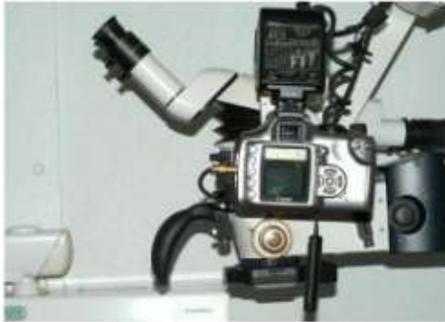
Fig. 32.16. Another view of the microscope of Fig. 32.14. The digital camera is connected with a strobe.
