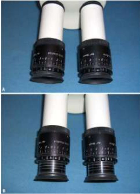
Fig. 32.25. Each eyepiece has several settings for the parfocal adjustment. Also, the position of the rubber cups may change: lower position if the operator is wearing glasses (A); raised position if the operator is not wearing glasses (B).
