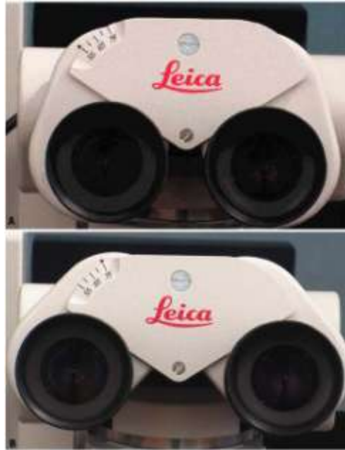
Fig. 32.23 A, B. The binocular allows to change the interpupillary distance in a range of 55 – 90 mm.
