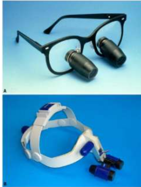
Fig. 32.5. A , Prism loupes. These loupes have sophisticated optics, which rely on internal prisms to bend the light (Courtesy of Designs for Vision, Inc, Ranonksima, NE, USA). B , The headset produced by Zeiss.
